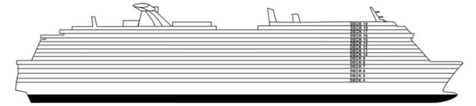
Gross Tonnage: 180,800 Length: 1130 feet Beam: 137 feet Cruising Speed: 17 Knots Guest Capacity: 5,270 (Double Occupancy) Total Staff: 1,735 Registry: The Bahamas
